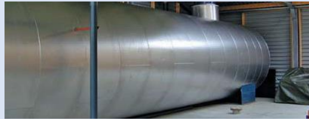
B: Plug flow digester made of stainless steel (Krieg and Fische Ingenieure, Germany)
